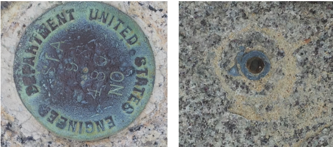
Figure 6: Left: US Engineering Department disk found in granite boulder located at the westerly end of the Cape Cod Canal north jetty. Right: Disk shaft and lead plug inserted into granite boulder in the jetty opposite the location of the 1940s US Engineering Department tide gage.
